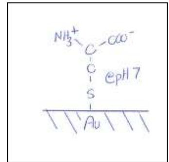
The cysteine will form a covalent sulfur-gold linkage with the electrode surface likely displacing any unwanted small molecules that have adsorbed to gold surface over time and stabilizing the impedance. This cysteine layer provides a hydrophilic substrate that is excellent for protein adsorption and ultimately cell attachment and spreading.
