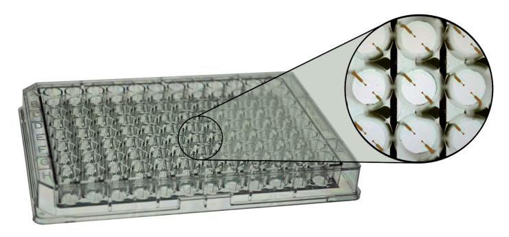
Each of the 96 wells in a standard plate configuration contains two circular 350 µm diameter active electrodes on a transparent PET substrate (measuring from 100-200 cells). As with other 1E arrays, a major use of this array is for the ECIS wound-healing assays where the small electrodes assures the high current pulse will result in complete cell killing.
