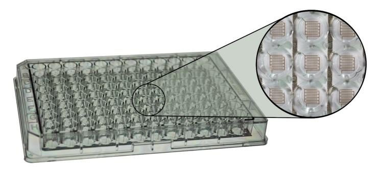
Each of the 96 wells has an Inter-digitated finger configuration. The total electrode area is  $3.985 \text{mm}^2$  which measures a maximum of 4000-8000 cells.
