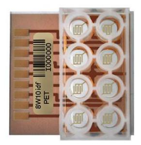
Our "mini" version of the 96W10idf array has 6 mm diameter wells for a substrate area of only 0.28cm<sup>2</sup> and a maximum well capacity of 200 microliters. The smaller well size means that less reagents and cells are required for experimental runs. The total electrode area is 2.09mm<sup>2</sup> which measures a maximum of 2000-4000 cells.
