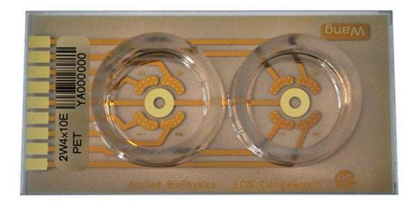
Each of the 2 circular 25 mm diameter wells contain four independent sets of ten 250 µm diameter active electrodes measuring from 2000-4000 cells. In addition, the 2W4x10E array is useful for duplicating readings in the same well or to wound/electroporate one electrode while leaving the other as a control within the same well.
