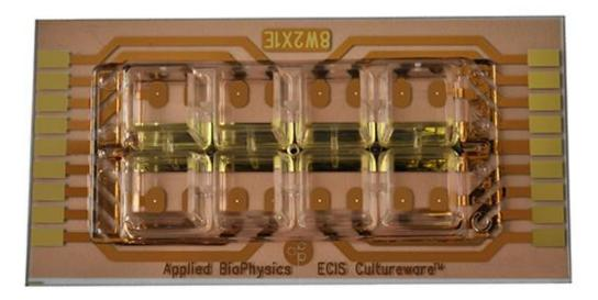
This array is also called the Medusa array. Each well in this array has two independent single 250  $\mu$ m diameter active electrodes. The Medusa array is useful for duplicating readings in the same well or to wound/electroporate one electrode while leaving the other as a control within the same well.
