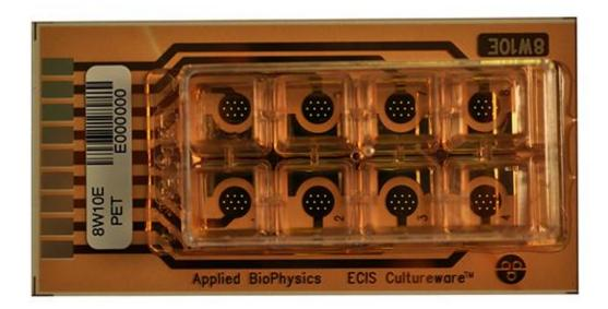
Each of the 8 wells contains ten circular 250  $\mu$ m diameter active electrodes connected in parallel on a common gold pad. Each well has a substrate area of 0.8 cm<sup>2</sup> and a maximum volume of 600  $\mu$ L. On average, with a confluent cell layer, approximately 500 to 1000 cells will be measured by the electrodes.
