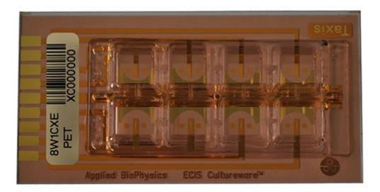
This array is used to monitor the movement of cells in response to chemical gradients and is the array used in chemotaxis measurements first described by Hadjout, N. et al. (2001) **Biotechniques 31** (5) 1130. The measuring electrode in this array is a thin gold line between two registry marks.\*
