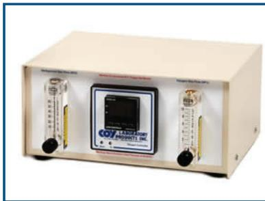
The oxygen controller has two ports, one for oxygen and the other for nitrogen/air (or a mixture of carbon dioxide and nitrogen/air). The system is designed to automatically maintain hypoxic or hyperoxic conditions in the cabinet with oxygen concentration from 0% to 60% (monitors up to 100%).
