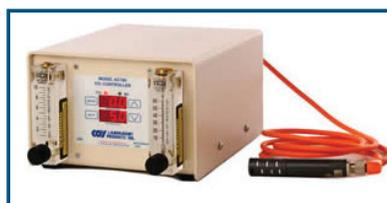
The carbon dioxide controller has two ports, one for CO<sub>2</sub> and one for nitrogen/air. The system regulates carbon dioxide concentration from 0% to 20% in single decimal increments using a gas purge method.
